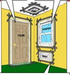
Duct tape plastic at corners first, then tape down all edges
